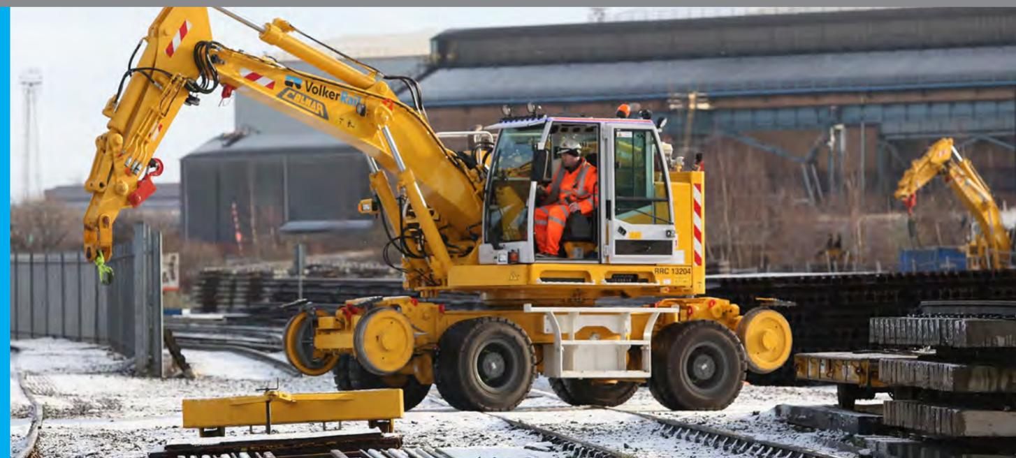
Rail mode – Level rail - Tool pin – unlocked - 0° - height 3m – Distance 5m = 10.97t
