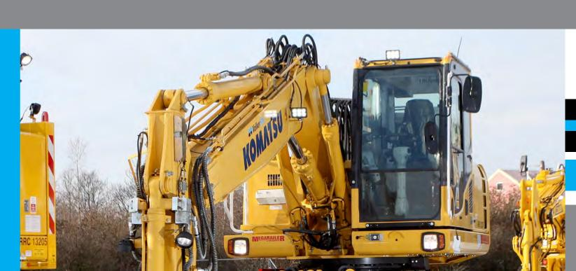
Machines are fitted with state of the art mr3 rail axle system. This Increases the machines lifting capacity, when undertaking lift and carry duties and unlocked duties are increased over oscillating axle.
