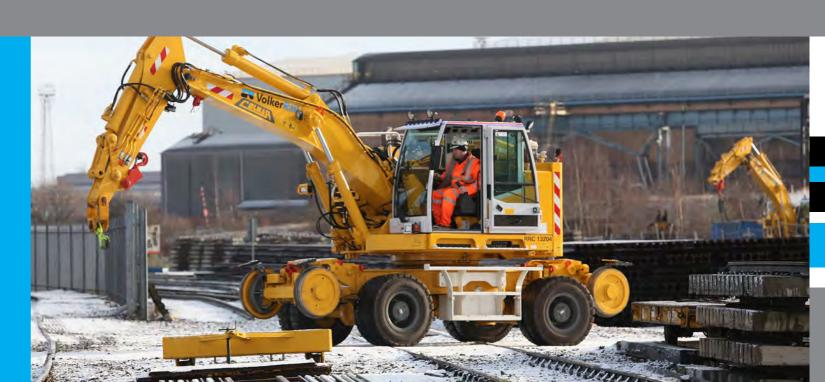
Rail mode – Level rail - Tool pin – unlocked -  $0^{\circ}$  - height 3m – Distance 5m = 10.97t
