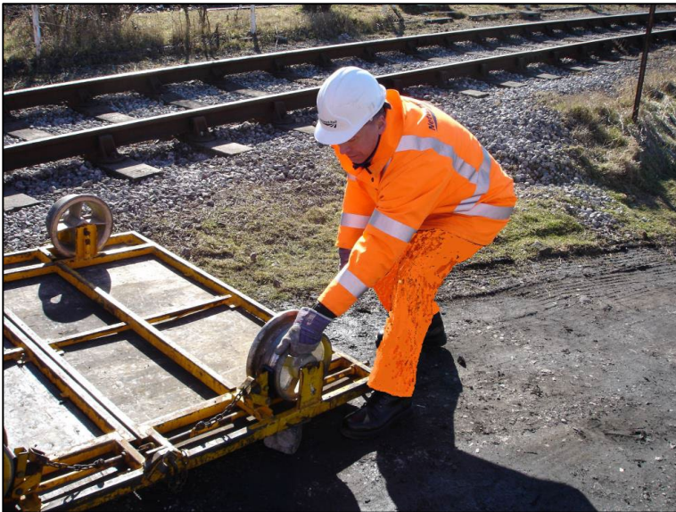
Figure 1 Checking Braked Wheels
